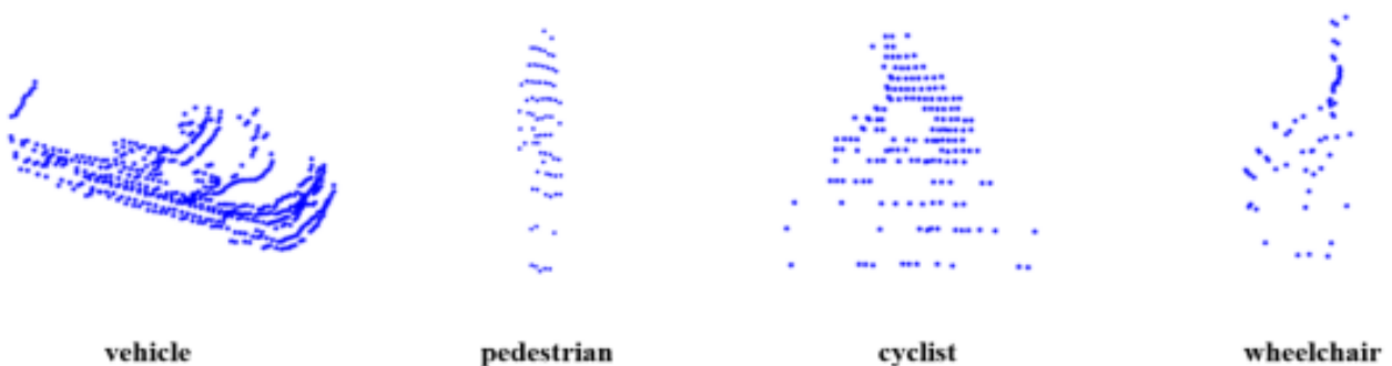
Figure A-33 - Examples of different road user clusters collected by 32-laser roadside LiDAR
